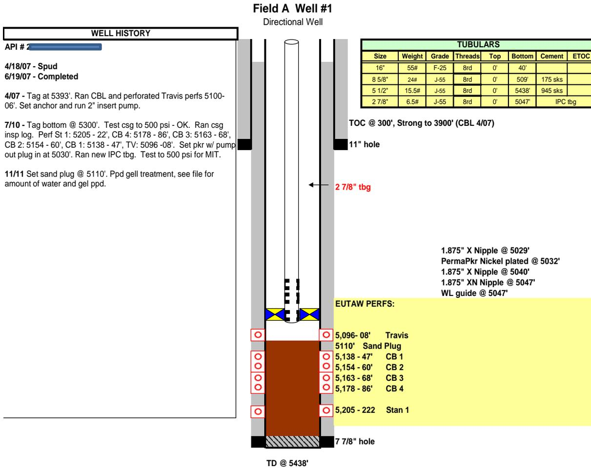
Figure 38. Wellbore Schematic for Field A, Well #1 Injector
