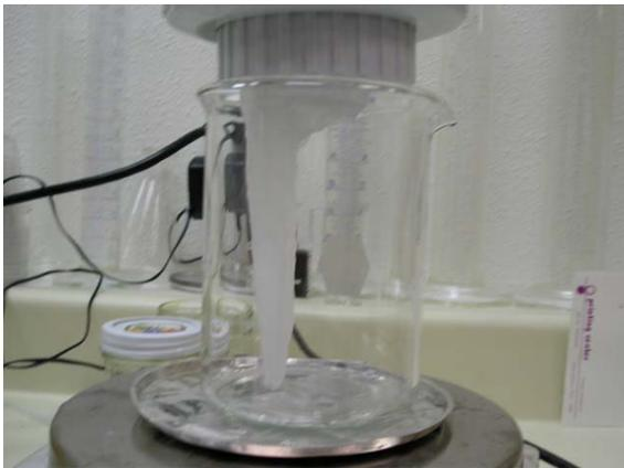
Figure 6. PAM cross-linked with Aluminum-Citrate tested through BGST
