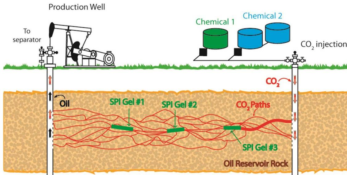
Figure 10. Schematic of Multiple, Smaller SPI Treatments in a Simplified CO<sub>2</sub> Flood
