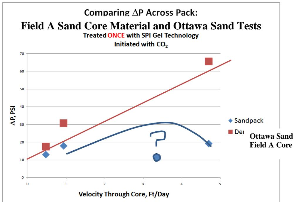
Figure 24. Field A Sandstone and Ottawa Sand Pack Water Injectivity Tests after 1<sup>st</sup> SPI Treatment
