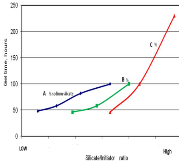
Figure 5. SPI Gel Time at 40°C versus Silicate/Initiator <sup>wt</sup> /wt Ratio
