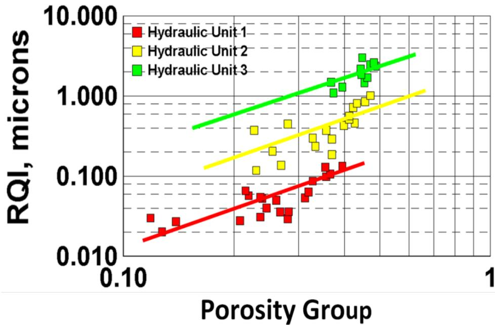
Figure 30. Plot Field A Reservoir Quality Index to Identify Hydraulic Units
