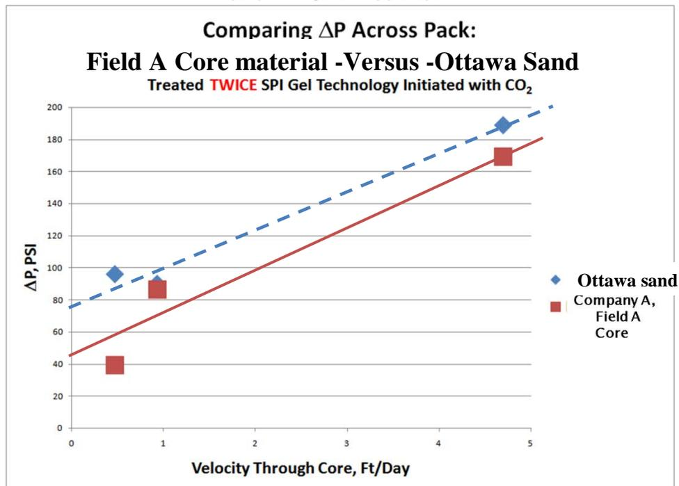
Figure 25. Field A Sandstone and Ottawa Sand Pack Water Injectivity Tests after 2<sup>nd</sup> SPI Treatment
